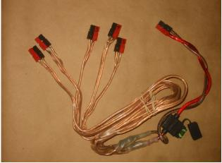
In my case, each arm of the Y is a different length, so I can connect various pieces of gear to the power supply without piling them on top of each other.
