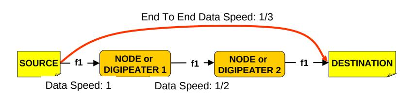
Data throughput is cut by a factor of 1 for each node/digipeater transition. The node/digi must receive the data and check that it is complete, then retransmit the data.
