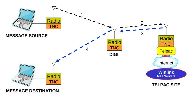
If it takes X minutes to send a message directly from the Source to the Destination, it will take 4X minutes if the message is sent via Winlink, through a digipeater. This means the frequency is not available for other use for 4X minutes.
