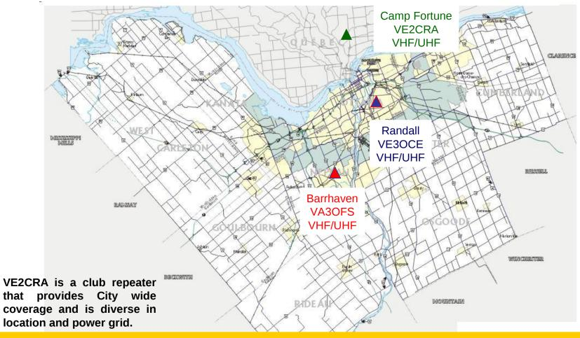
There is no single repeater that can cover the full City of Ottawa. By using several repeaters, most areas are covered and are accessible from key locations.
